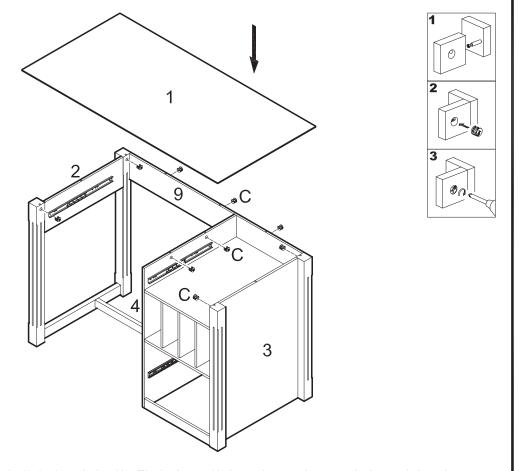
Insert cam locks (C) into panels (2,3,4) and slat (9). Fit desk top (1) into place using cam bolts and dowels as guides. Tighten cam locks (C) with a screwdriver to secure desk top (1).
