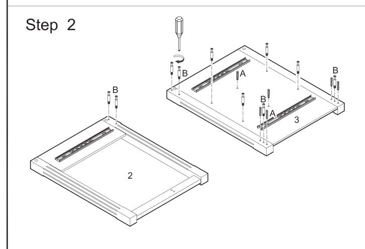
Insert dowels (A) into panel (3). Screw cam bolts (B) into panels (2,3) with a screwdriver.
