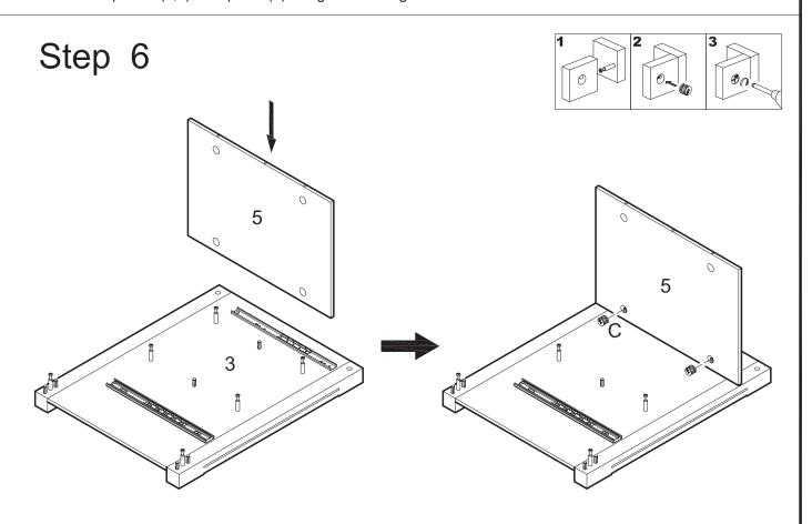
Fit panel (5) onto panel (3) using cam bolts and dowels as guides. Insert cam bolts (C) into panel (5) and tighten with a screwdriver.
