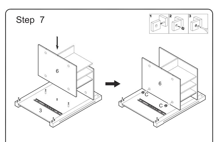
Fit panel (6) with divider panels onto panel (3) using cam bolts and dowels as guides. Insert cam locks (C) into panel (6) and tighten with a screwdriver.
