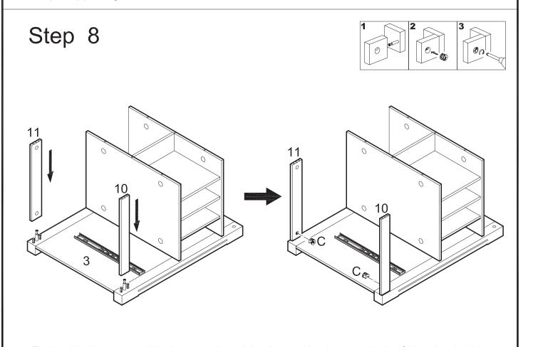
Fit slats (10,11) onto panel (3) using cam bolts and dowels as guides. Insert cam locks (C) into slats (10,11) and tighten with a screwdriver.
