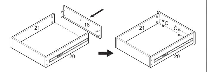
Fit drawer front (18) onto drawer sides (20,21) using cam bolts as guides. Insert cam locks (C) into drawer sides (20,21) and tighten with a screwdriver.
