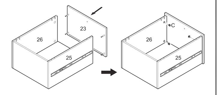
Fit drawer front (23) onto drawer sides (25,26) using cam bolts as guides. Insert cam locks (C) into drawer sides (25,26) and tighten with a screwdriver. *Note that two cam locks will be inserted into each drawer side*.
