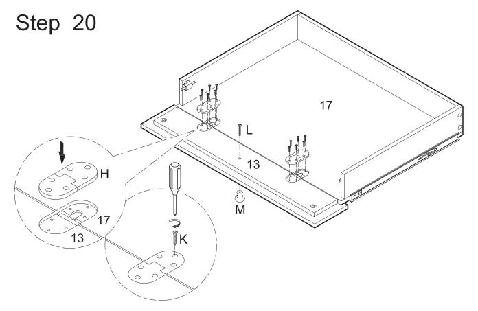
Align drawer front (13) with drawer bottom (17). Place hinges (H) into the slots of drawer pieces (13,17) and attach them to the drawer pieces using screws (K). Attach knob (M) to drawer front (13) using bolt (L). Tighten screws (K) and bolt (L) with a screwdriver.
