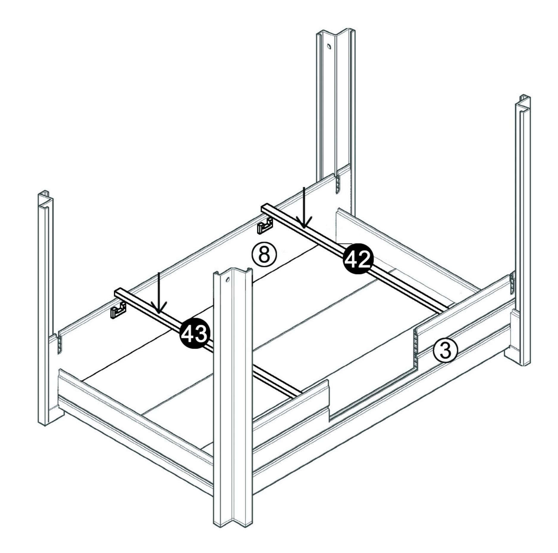
Note: If you chicken barn comes with 2 roosting bars. Put the roosting bars 42 and 43 into the U-shaped slots on wall panels 3 and 8.
