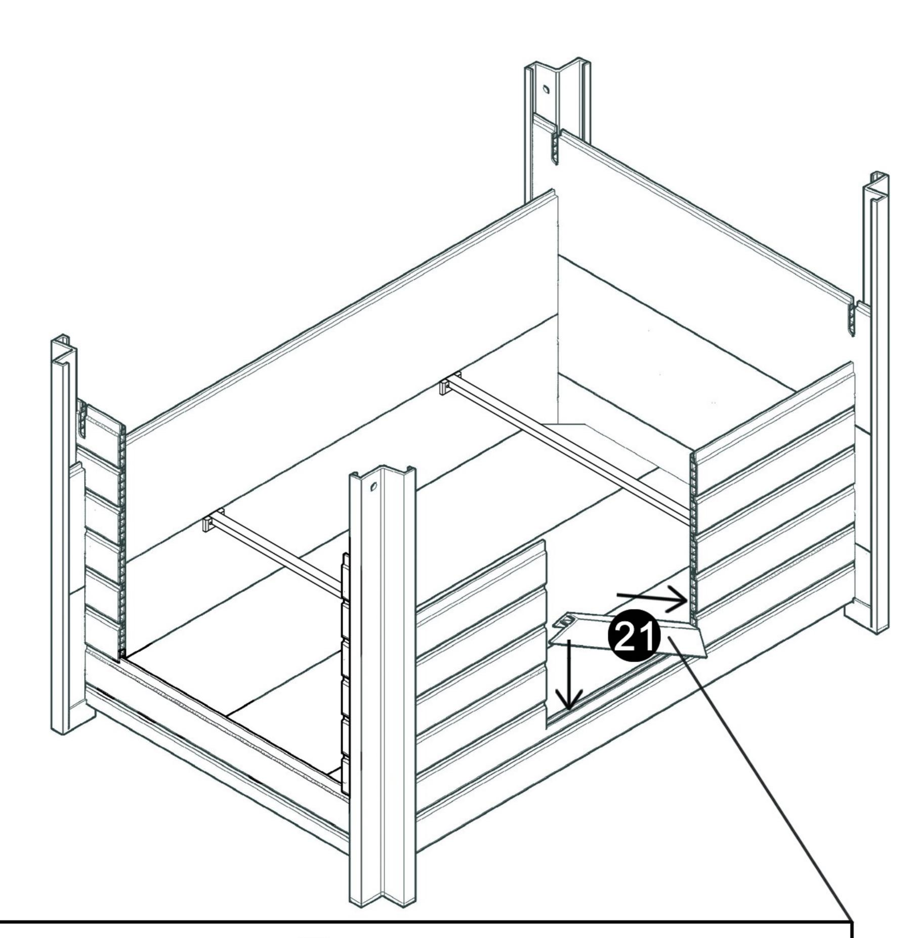
Place door frame 21 into one of the lower corners of the door opening, then push the other end down gently. The side of the frame piece with part # bar code should be facing inside the barn. Same for all door frame pieces.
