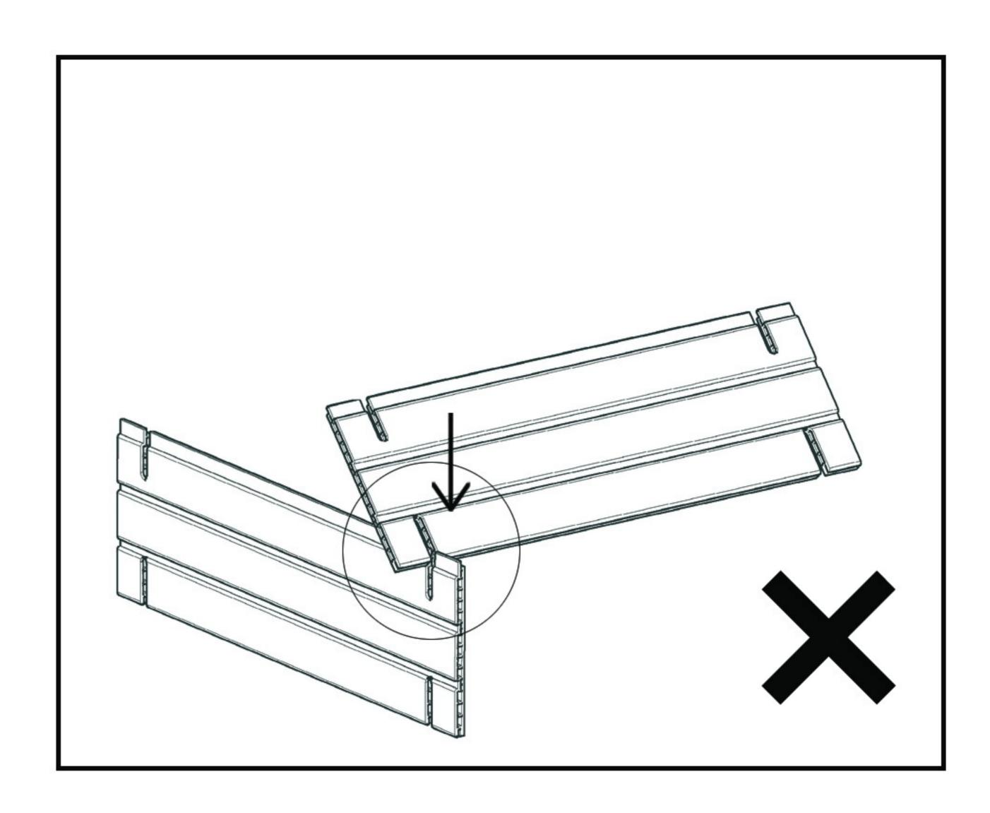
When installing wall panels, make sure the two connecting panels are at a 90 degree angle vertical to the ground, and 90 degree perpendicular to each other. Tilting in any way might cause damage to the groove.
