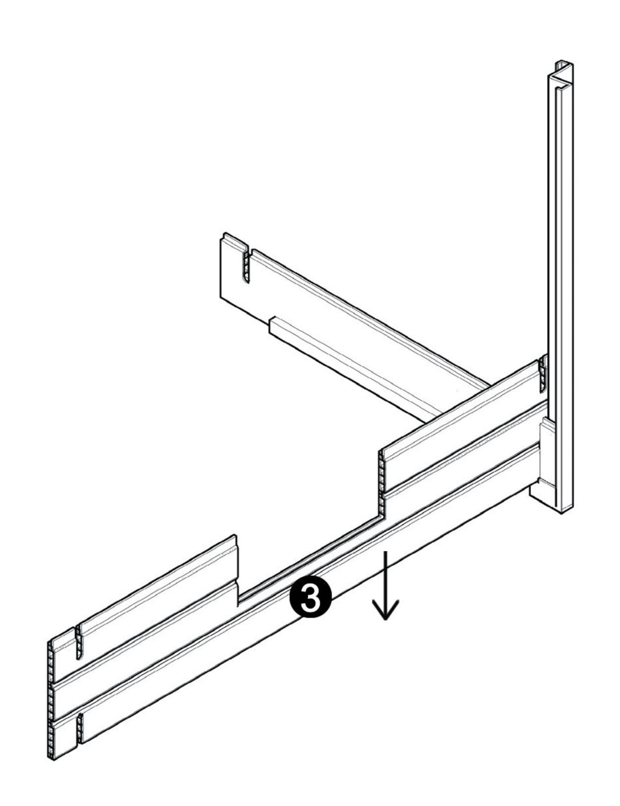
Note: After install Panel 3, make sure the FLAT side of panel 1 and 3 are facing inside, and the washed sides are facing out.
