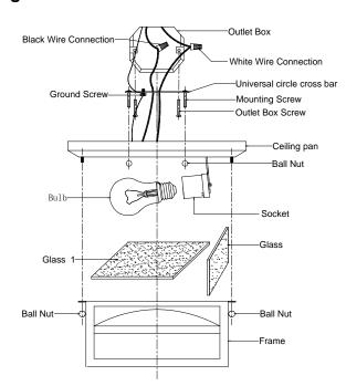
STEP 6: Install the glass panels into the frame, and then combine the fixture with the frame, and fasten it with the ball nuts.
