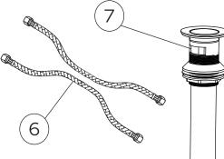
Note: This faucet has been packaged with an over-flow pop-up drain. DO NOT use with a non-over-flow sink.
