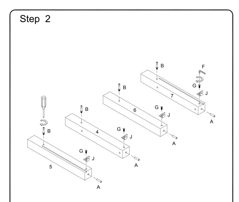
Attach cam bolts (B) to parts (4,5,6,7) using Phillip's head screwdriver. Then attach bracket (J) to parts (4,5,6,7) using bolts(G) and hex key (F) as per diagram.
