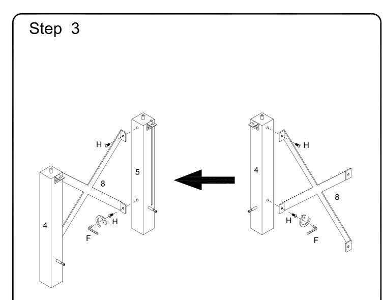
Using bolt (H) secure part (8) to part (4) ,then secure to part (5) as per diagram.
