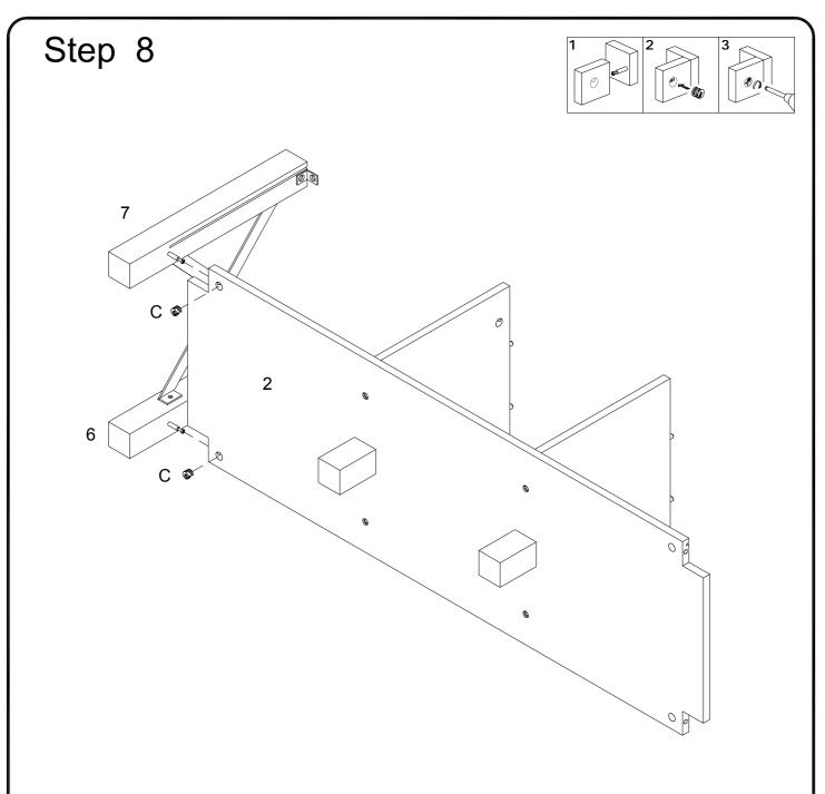
Using cam lock (C) connect part (2) to parts (6,7) as per diagram.
