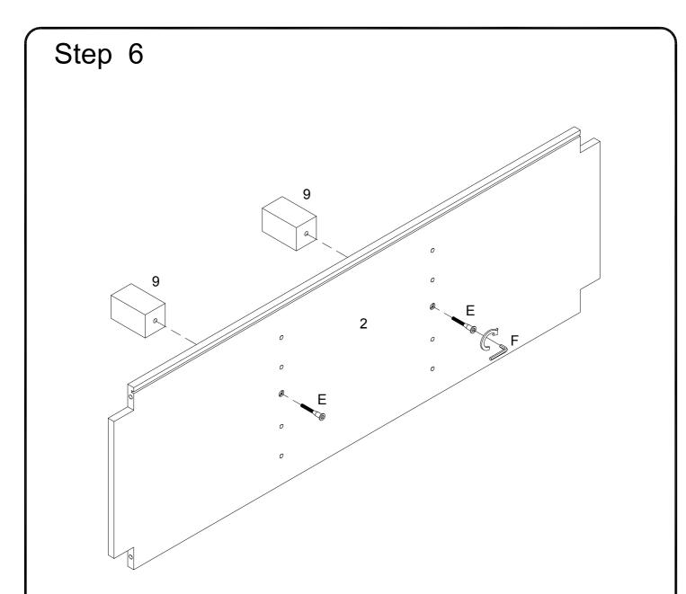
Attach part (9) to part (2) using screw (E) and hex key (F).
