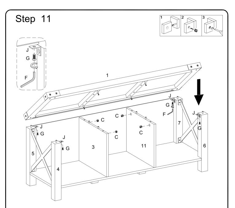
Put part (1) to parts (3,4,5,6,7,11) ,and using bolt (G) secure L shape bracket (J) with hex key (F) as per diagram .
