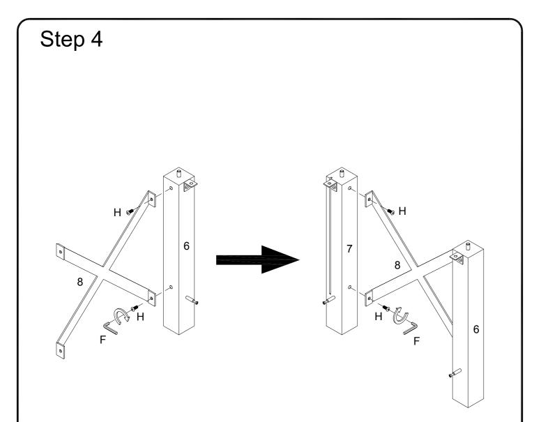
Using bolt (H) secure part (8) to part (6) ,then secure to part (7) as per diagram.
