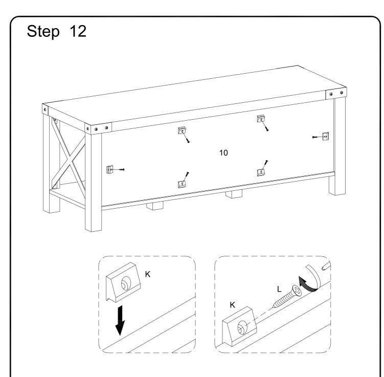
Using screw (L) secure plastic wedge (K) to part (10) with Philips head screwdriver as per diagram.
