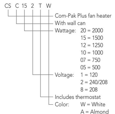
If horizontal mounting is preferred for heater assemblies without thermostat, use model CMGA or CMGW.
