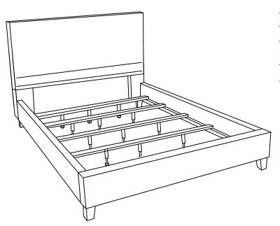
This page lists all the contents included in the box. Please take the time to identify the hardware as well as the individual components to this product. As you unpack and prepare for assembly, place the contents on a carpeted or padded area to protect them from damage. Attached Wooden Leg(C) to the Footboard(A) use Bolt(G), Lock Washer(J) and Flat Washer(I) on both of holes. Turn the Allen Wrench(K) in Bolt(G).
