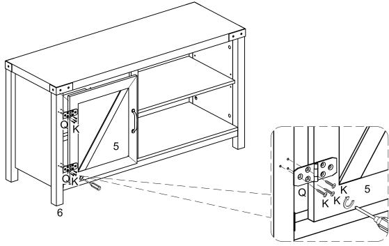
Attach part (5) to part (6) to secure hinge (Q) using screw (K) with screwdriver.
