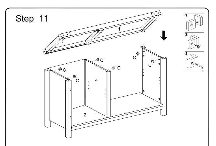
Attach part (1) to part (3,4) then insert and secure cam lock (C) to part (3,4) to lock it.
