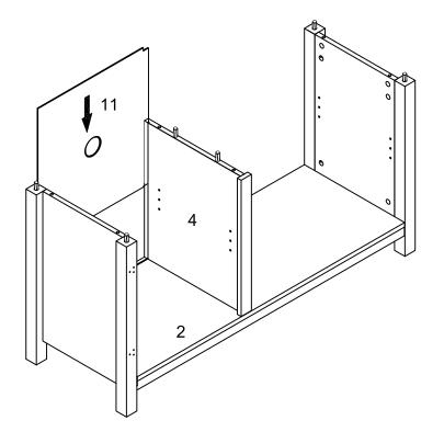
Slide back panel (11) into grooves as per diagram.
