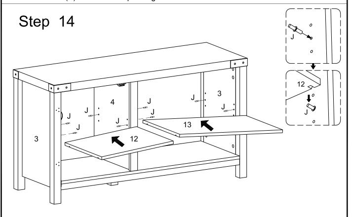
Insert shelf support pin (J) into side panel (3,4), then place shelf (12,13) on top of support pin (J).
