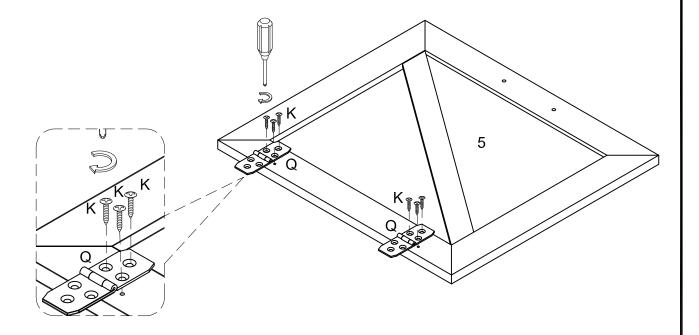
Attach hinge (Q) to part (5) using screw (K) with screwdriver.
