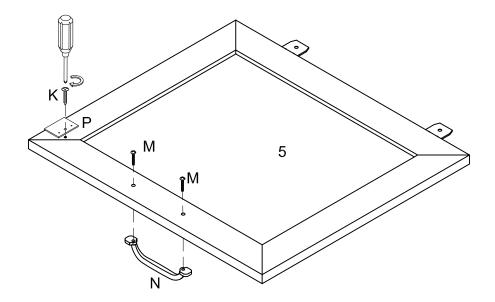
Attach door plate (P) using screw (K), handle (N) using bolt (M) to part (5) with screwdriver.
