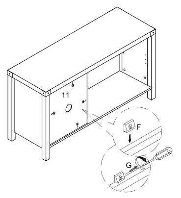
Attach plastic wedge (F) to part (11) using screw (G) with screwdriver.
