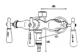
\*The minimum center to center of 4 1/2" when mounting on a "bathroom wall" AND/OR any faucet that has P0166 swing arms added for wall mount installation.
