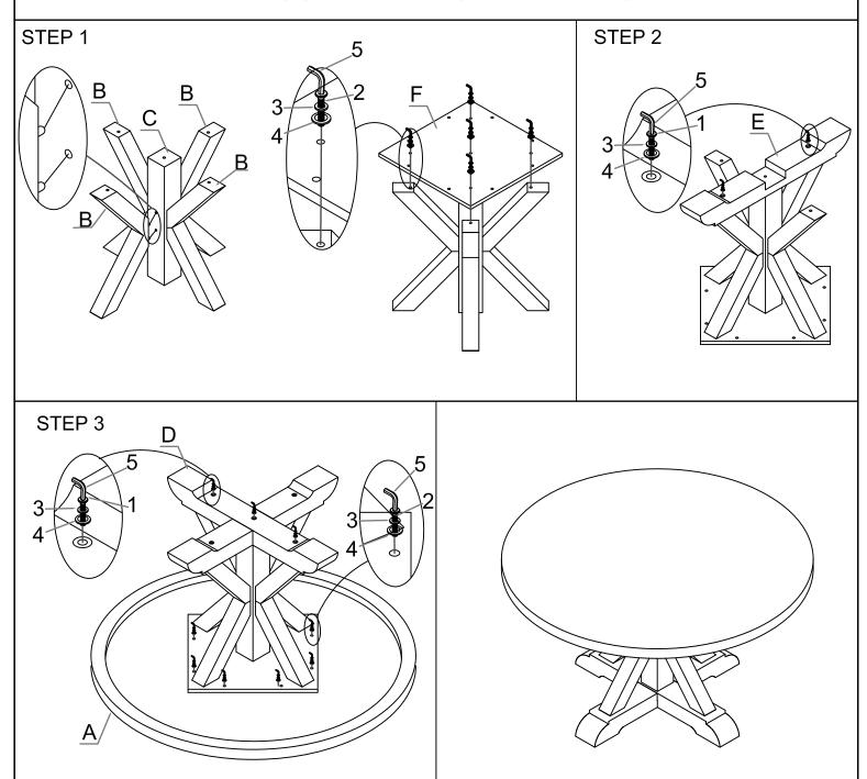
**Step 1:** Attach Leg (B) to Connecting Wood (C) and assemble Mounting Plate (F) by inserting Flat Washer (4), Spring Washer (3), Short Bolt (2) into the holes on the Mounting Plate (F) to the Leg (B) and Connecting Wood (C). Tighten Short Bolt (2) with Allen Key (5). Do not fully tighten.
