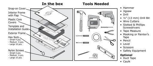
NOTE: The Extreme Weather Pet Door can be installed in most doors and walls. Installation in thinner or thicker applications may not require the Plastic Core Covers. If installing in a wall, reduce cut-out width by 1" for the Small and Medium. For the Large reduce cut-out width by 1" and cut-out height by 1". Additional tools and materials, such as wood framing, may be required.
