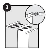
Remove screws, insulated flap and backing plate from back of flap clamp. Insert new insulated flap between flap clamp back and backing plate. Align screw holes. Replace and tighten screws. Follow step 3 under "Vinyl Flap Replacement and Adjustment" on page 9.
