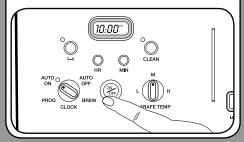
To Program the Auto Off: Turn the Function knob to AUTO OFF. Follow Set the Time instructions to program Coffeemaker to shut off 0 to 4 hours after brew cycle is finished.
