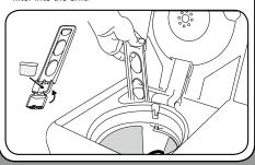
Pour desired amount of water into water reservoir (a water level indicator is located on the side of the unit).
