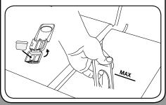
Fill the water reservoir with cold water to the maximum fill line.
