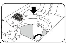
Check to make sure the filter basket is securely in place and lid is completely closed.
