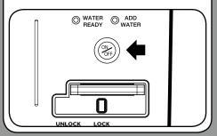
Move safety switch left to unlock. Place a cup on drip tray and press the lever down. The unit will dispense 10 oz. of hot water at a time. **NOTE:** Hot Water System works independently of Coffeemaker; it can be filled and heated before, during, or after coffee is brewing.
