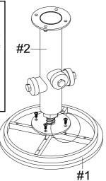
2) Attach the base (#2) with the seat panel (#1) by screwing in the bolts (#A) with the allen wrench M4 (#C).
