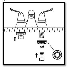
4. Connect to Water Supplies (Hook-Ups Not Provided). Flush System/Check for Leaks Connect the hot and cold water supplies to the shanks as shown. Remove the aerator. Turn the handle all the way on. Turn on hot and cold water supplies and flush water lines for one minute. This flushes away any debris that could cause damage to internal parts. Check all connections for leaks. Replace aerator. Retighten if necessary, but do not over tighten.
