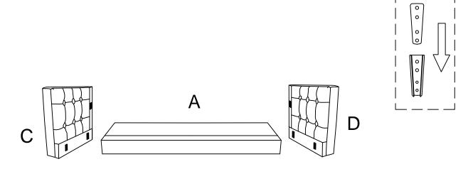
Hook on the Back (B) to Left Panel (C) & Right Panel (D) properly.
