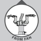
Using orange wire connectors from the hardware bag, connect the black wire (ungrounded) from the ceiling to the black and the blue wires from the fan. Connect the white wire (grounded) from the ceiling to the white wire from the fan.
