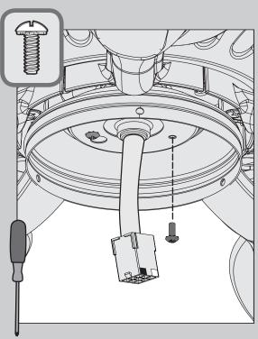
Insert the third screw, found in the ≡ hardware bag, into place and then tighten all three (3) screws.
