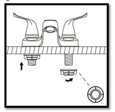
**Connect to Water Supplies (Hook-Ups Not** 4. Provided). Flush System/Check for Leaks Connect the hot and cold water supplies to the shanks as shown. Remove the aerator. Turn the handle all the way on. Turn on hot and cold water supplies and flush water lines for one minute. This flushes away any debris that could cause damage to internal parts. Check all connections for leaks. Replace aerator. Retighten if necessary, but do not over tighten.
