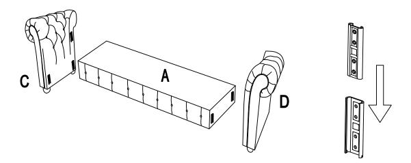
Hook on the Back Frame (B) to Left Panel (C) & Right Panel (D) properly.
