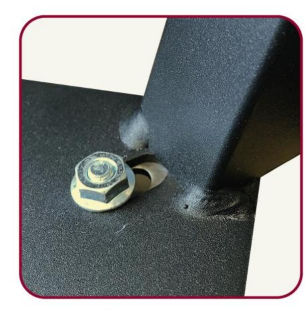
Support base spot welded (1 side) to legs. Partial contact (legs to plate).
