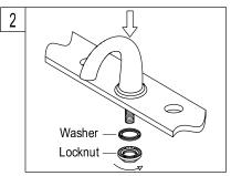
2. Install new faucet spout through the center hole of sink. Place mounting washer on spout shank and attach with spout shank locknut.
