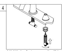
4. Hold the handles in proper position. Make sure that the top of the faucet handles is 5/8" above the top of the sink. Mount the metal washer and locknut from underneath the sink. Than reposition escutcheons as necessary to a desired height.
