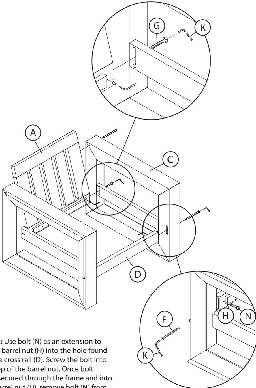
**NOTE:** Use bolt (N) as an extension to insert barrel nut (H) into the hole found on the cross rail (D). Screw the bolt into the top of the barrel nut. Once bolt (F) is secured through the frame and into the barrel nut (H), remove bolt (N) from barrel nut (H).
