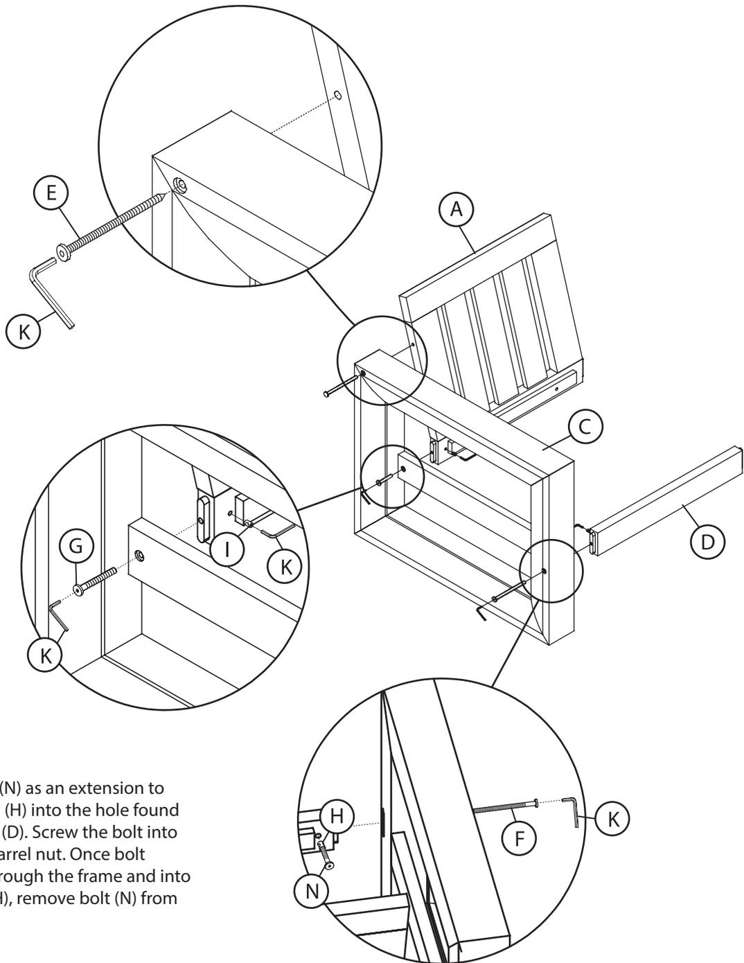
**NOTE:** Use bolt (N) as an extension to insert barrel nut (H) into the hole found on the cross rail (D). Screw the bolt into the top of the barrel nut. Once bolt (F) is secured through the frame and into the barrel nut (H), remove bolt (N) from barrel nut (H).
