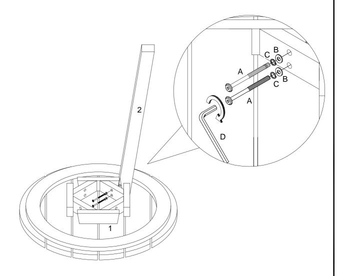
Fasten part (2) to part (1) by using bolt (A) with lock washer(C) and flat washer(B) with hex key (D)
