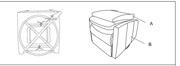
Carefully cut the strips on the bottom of seat with a pair of scissors. Remove Chair Backrest(A) from the Chair Base with Footrest(B).
