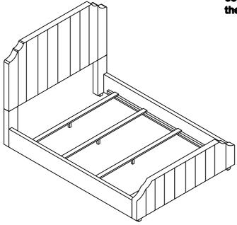
ATTACHED FOOT BOARD(B), LEG(F), FLAT WASHER(K), LOCK WASHER (I),BOLT(H), BY ALLEN WRENCH(L).
