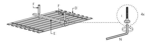
Spread the Slats (D) and place it to the Side Rail (G). Tighten the Slats (D) with CSK Screw (M) using Philip Head Screwdriver (Not provided).
