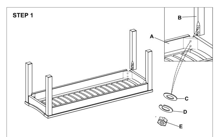
Attach the leg frames (B) into each corner of the top (A). Assemble the washers (C), spring washers (D) and nuts (E) to leg frames (B). Tighten the nuts using wrench.
