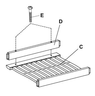
Attach the apron (D) into bottom of seat (C) and secure using 2 1/4" bolts (E).
