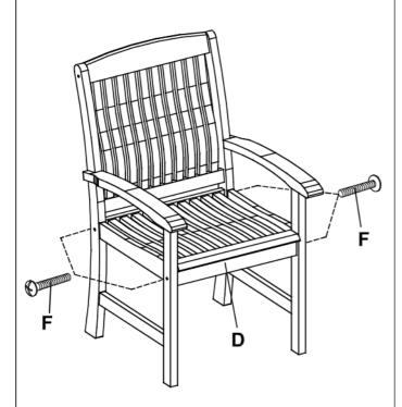
Next, attach the pre-assembled seat into right and left side frames (A1 & A2). (The seat with apron must be attached in front). Secure seat using 1" bolts (F) as shown. Tighten all bolts using screwdriver.
