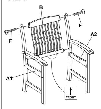
Attach right and left side frames (A1 & A2) into back support (B). Secure using 1" bolts (F).
