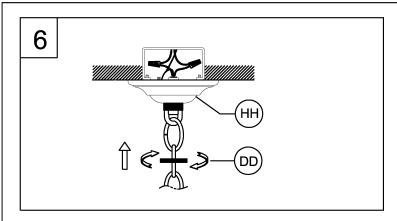
6. Tuck the wires into the junction box and slip the canopy over the chain holder. Thread the screw collar (DD) onto the chain holder to secure the canopy tightly to the ceiling.
