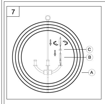
7. Place candle cover (B) and candle cap (C) onto fixture socket. Screw lamp (not included) into fixture socket. Use 60-watt MAX incandescent candelabra base, SBCFL or SBLED.
