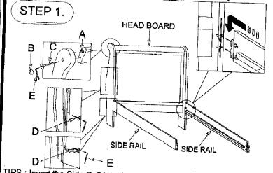
TIPS: Insert the Side Rail into the hole of Headboard.
