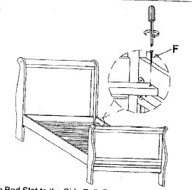
TIPS: Attach the Bed Slat to the Side Rail. Fasten the Bed Slat by tighten with Screw M4 x 32mm through the pre-drilled hole of Bed Slat
