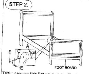
TIPS: Insert the Side Rail into the hole of Footboard.
