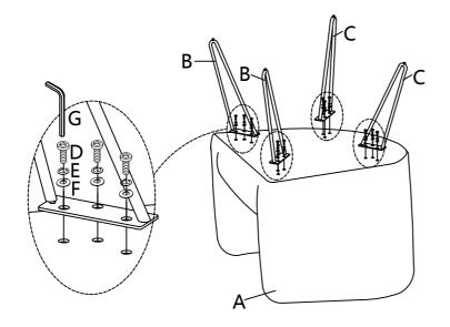
Take the Allen Wrench, and turn the bolts until the legs are secured. DO NOT TIGHTEN COMPLETELY. Stop when you feel you are adding force to tighten the bolt.
