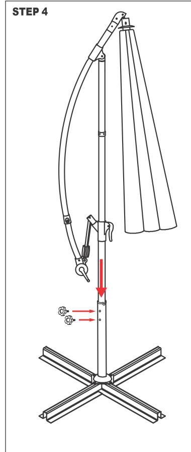
Firmly insert the Umbrella into the assembled base. Screw in and tighten the Threaded Knobs into the pole support.
