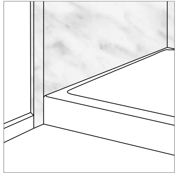
Vertical trims installed outside shower base
