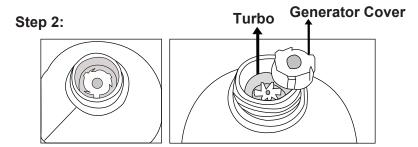
Remove the Generator Cover. Clean the Turbo and turn the Turbo a couple turns.
