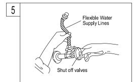
5. Connect the water supply lines. Before connecting the supply lines, apply pipe joint compound to the threads on the inlet shanks and shut off valves with an adjustable wrench.
