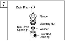
7. Install flange body up through the drain opening, hold the drain flange body in position with pivot rod opening facing the back of sink and hand tighten the mounting nut.
