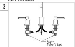
Apply Teflon's tape to inlet shanks and connect supply lines.
