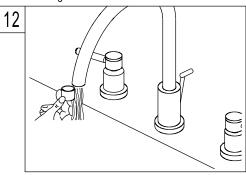
12. Remove the aerator before turning on your new faucet for the first time, let hot and cold water run for at least 1 minute, replace aerator this will prevent debris in the line from clogging the aerator.
