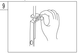
With lift rod in position on the faucet, insert lift rod through lift rod strap and secure with the clevis screw.
