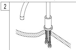
Install new faucet spout through the center hole of sink. Place mounting washer on spout shank and attach with spout shank locknut.
