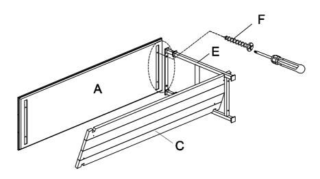
Attach another Side Frame (E) to the Top Panel (A) by using Bolt-Small (F), fixing the Bottom Panel (C) to Side Frame (E) by using Bolt-Big (G), and then attached the Spacer (I) to the bottom of the Side Frame (E).
