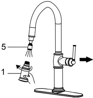
Remove spray head (1) from spray hose (5). Hold tip of spray hose (5). Turn faucet on and let the water run for 60 seconds to flush any debris.
