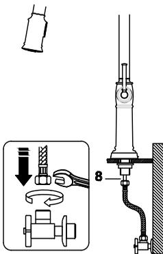
Connect waterlines (8) to angle stops. Tighten both ends of waterlines with a wrench until snug. Turn on hot and cold angle stops and check for leaks.
