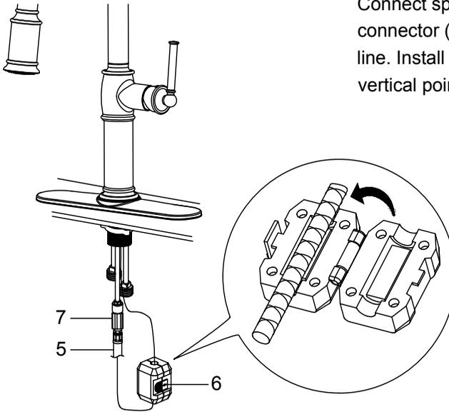
Connect spray hose (5) to quick connector (7) attached to supply line. Install weight (6) on lowest vertical point on spray hose (5).
