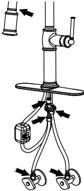
Check for leaks at the connections. Retighten if necessary.
