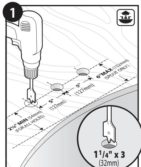
Drill holes in rough or finished deck for the valves and spout 5" minimum on center. Position the spout hole so that spout delivers the water to the desired place in the tub.
