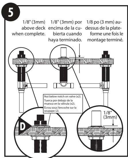
When properly assembled, top nuts (D) are below notch on each valve. On center shank, leave 1/8" of threads above deck.
