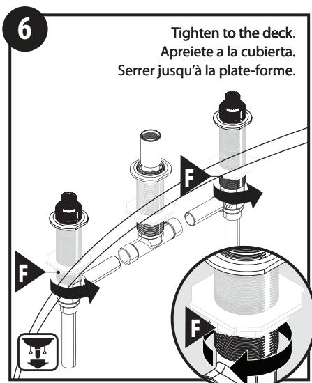
Secure valves & shank, tighten lower nut firmly using pliers.
