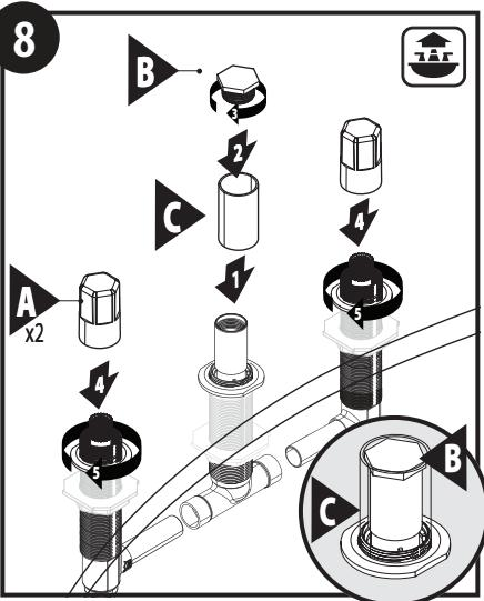
Place protective tube (C) over center shank assembly (I) and protective caps (A) over valves (G & H). Secure protective tube (C) with test plug (B).
