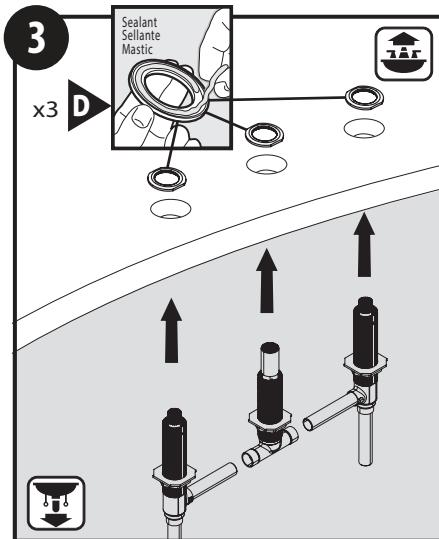
From the underside of the deck, insert completed assemblies. Add bead of sealant on bottom of top nuts.
