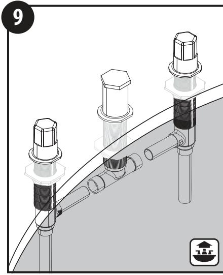
Solder all connections, then check for leaks.
