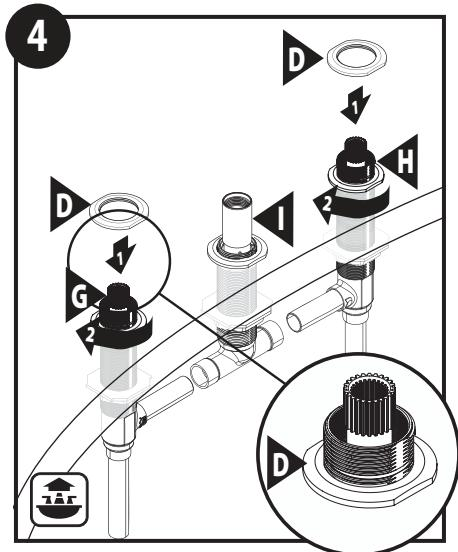
Thread top mounting nuts (D) on each valve (G & H) and spout shank (I).
