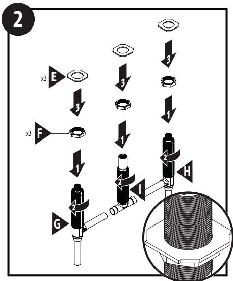
Assemble nut (F) and washer (E) onto valves (G & H) and onto shank assembly (I).
