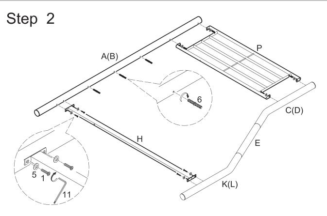
Screw double-sided screws (6) into post (A). Attach guardrail (P) to post (A) and curved post section (C) using medium bolts (1) with small washers (5). Attach crossbar (H) to post (A) and curved post section (K) using medium bolts (1) with small washers (5). Tighten medium bolts (1) with small wrench (11). Repeat this step with post (B) and curved post sections (D,L) on the opposite side of the bunk bed.
