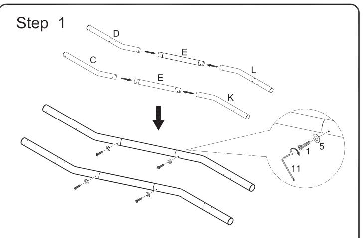
Slide curved post sections (C,K) and curved post sections (D,L) onto post sections (E). Secure the post sections together using medium bolts (1) with small washers (5). Tighten medium bolts (1) with small wrench (11).
