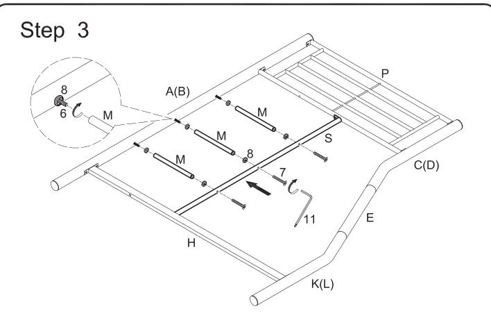
Slide washers (8) onto double-sided screws (6). Screw ladder rungs (M) onto double-sided screws (6). Attach ladder rail (S) to ladder rungs (M) using bolts (7) with washers (8). Tighten bolts (7) with small wrench (11). Repeat this step on the opposite side of the bunk bed.
