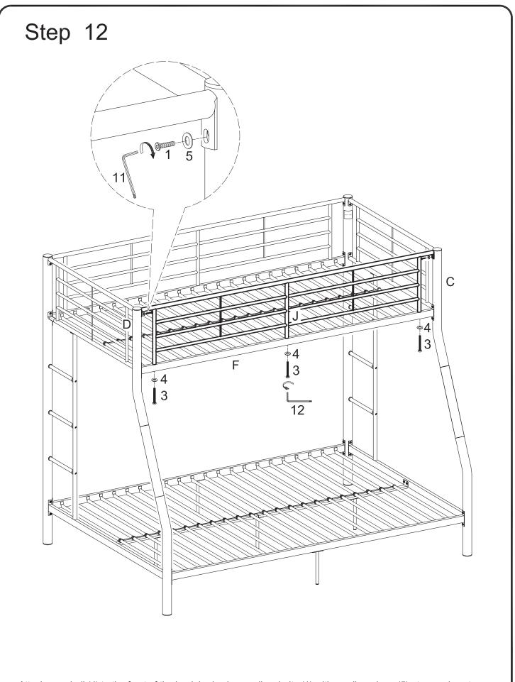
Attach guardrail (J) to the front of the bunk bed using medium bolts (1) with small washers (5) at curved post sections (C,D), and large bolts (3) with large washers (4) at crossbar (F). Tighten all bolts with wrenches (11,12).
