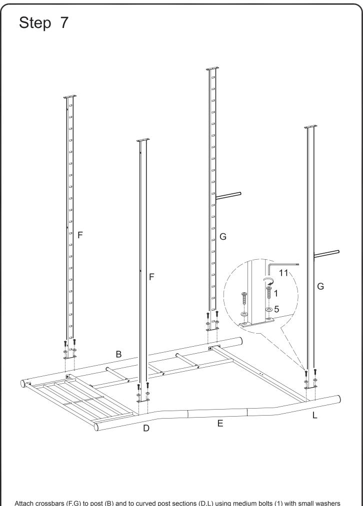
Attach crossbars (F,G) to post (B) and to curved post sections (D,L) using medium bolts (1) with small washers (5). Tighten medium bolts (1) with small wrench (11).
