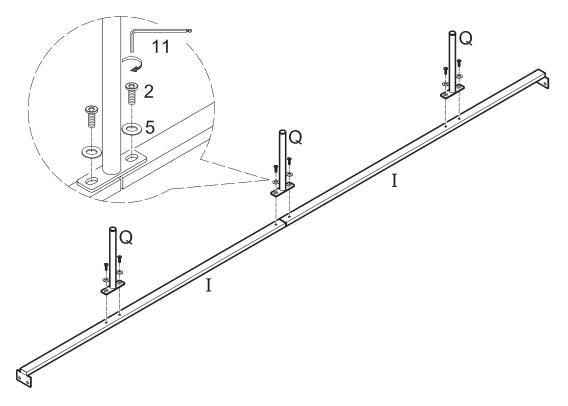
Attach support legs (Q) to support bars (I) using small bolts (2) with small washers (5). Tighten small bolts (2) with small wrench (11).
