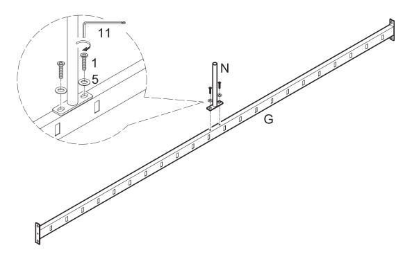
Attach support leg (N) to crossbar (G) using medium bolts (1) with small washers (5). Tighten medium bolts (1) with small wrench (11). Repeat this step for second crossbar (G).
