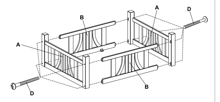
Attach side frames (A) into side frames with metal clip (B) as shown. Secure using 2 1/4" bolts (D) and tighten all bolts using screwdriver.
