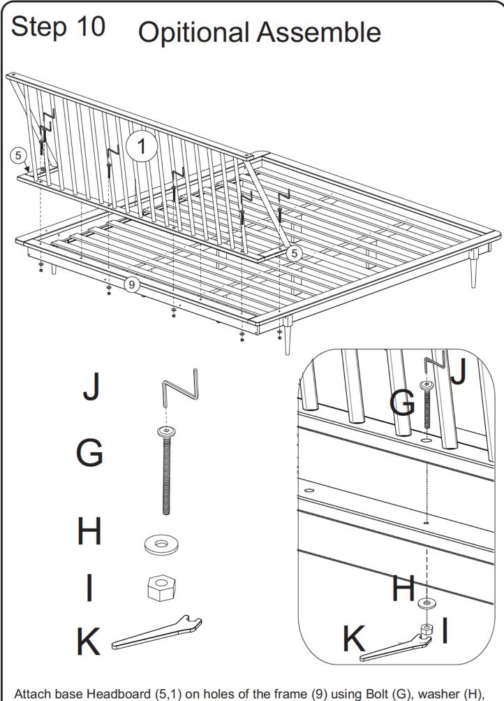
Attach base Headboard (5,1) on holes of the frame (9) using Bolt (G), washer (H) and nut (I) Tighten using both the hex key (J) and wrench(K)
