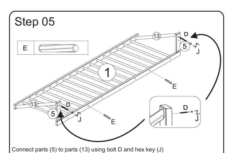
Insert Wood Dowel (E) in holes to part (1)
