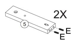
Insert wooden dowels (E) into rails (5), dowels (F) into parts (13),
