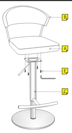
In order to activate the gas hydraulic, it is important that once you have assembled the stool that you raise the lever and bounce your weight up and down on the stool and then lift your weight off with the lever still raised and the stool should begin to
