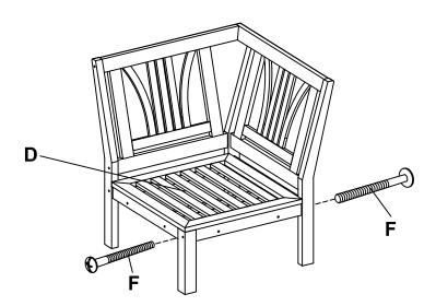
Next, attach the seat (D) into pre-assembled of side frames and secure using 2 1/4" bolts (F). Make sure all parts are correctly connected and tighten all bolts completely. Repeat step 1 and 2 procedure to secure other corner chairs.
