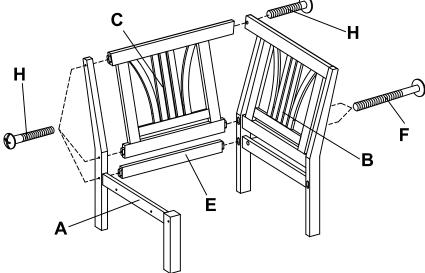
Attach side frame (A) and side frame with support (C) into back support (B) and apron (E). Secure using 1 1/2" bolts (H) into side frame (A) and 2 1/4" bolts (F) into side frame with support (B) as shown.
