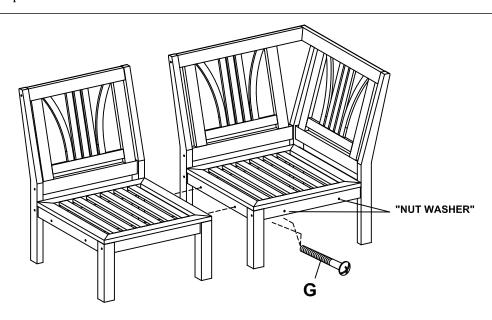
Next, joint the corner chair with other chair and secure using 2" bolts (G) from underneath of seat.
