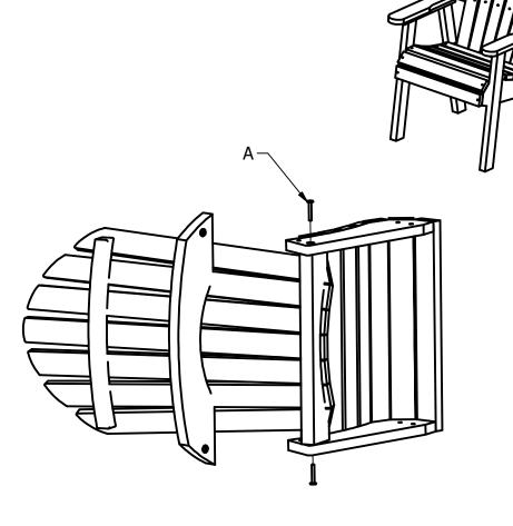
**1)** Insert an A bolt into lower hole to on each side attach Seat to Back. Make sure the back is fully upright. Make bolts snug, but do not overtighten.
