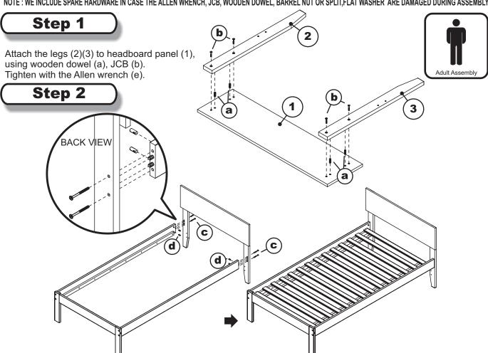
Attach bed frame assemblies to the headboard assemblies, using JCB M6 X 70mm (c) and barrel nut (d) as shown. Tighten with allen wrench (e). For Slat kit assembly, follow assembly instructions included with slat kit.
