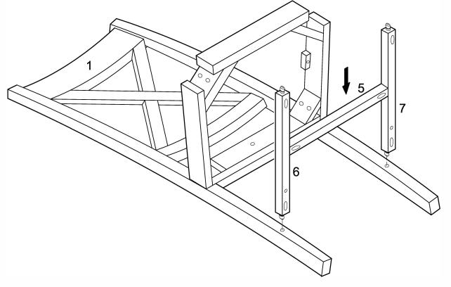
Attach crossbars (6,7) with crossbar (5) to chair back (1) using dowels as guides.
