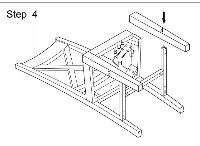
Attach legs (3,4) to the chair assembly using bolts (B), spring washers (D) and washers (E). Tighten all bolts (B) with wrench (H).
