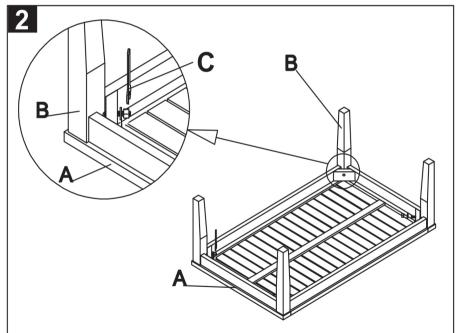
Step 2: tighten all bolts to the support of the table top by using the wrench(C).
