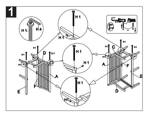
Step 1: attach right side (D) to the back (A). Then attach support L (E) and support S (F) to the right side (D) as shown on the picture by using the Allen Bolt (H1) and tighten all with the Allen Key (H4). Continue with the left side (C) in the same way. Make sure to tighten all bolts (H1) before you continue with step 2.
