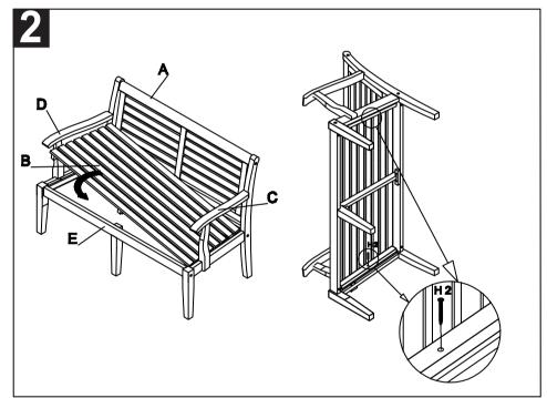
Step 2: put the seat (B) inside the bench as shown on the picture and use the screws (H2) to attach it to the chair by using a screwdriver.
