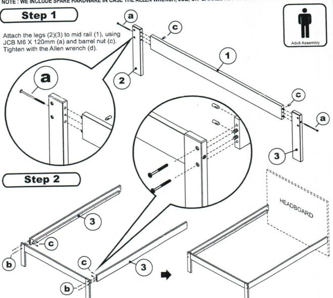
Attach long rail (3) to the mid rail assemblies, using JCB M6 X 70mm (b) and barrel nut (c) as shown. Tighten with allen wrench (d). For Headboard assembly, follow assembly instructions included with headboard. Page 1 of 1
