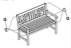
Tapping in the wooden caps (G) to cover bolts head using rubber mallet.
