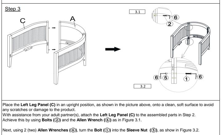
Do not fully tighten the Bolts at this time.
