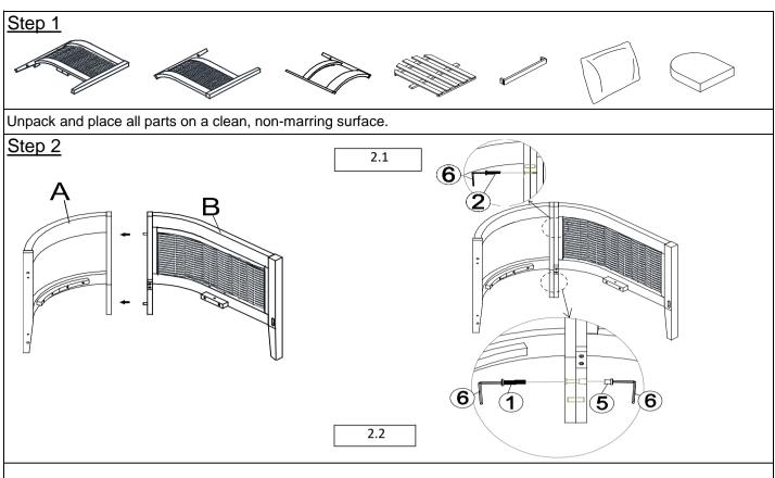
Place the **Backrest Panel (A)** in an upright position, as shown in the picture above, onto a clean, soft surface to avoid any scratches or damage to the product.
