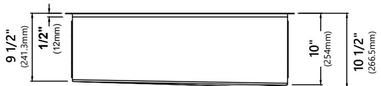
**NOTE:** It is not recommended to install this sink with a negative reveal. Doing so will prohibit the use of any workstation accessories as they will not fit.
