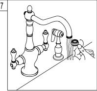
7. Remove the aerator before turning on your new faucet for the first time. This is to prevent any deposits from clogging your aerator. Allow both hot and cold water to run for one minute. Replace aerator.
