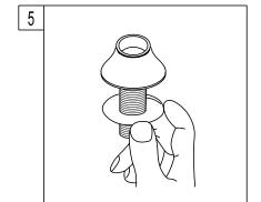
5. For model is with spray head and hose. Place the spray guide through the fourth hold in the sink, screw the locknut onto the shank and tighten firmly.
