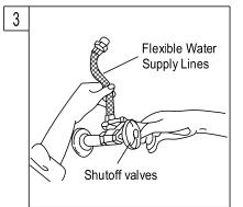
3. Connect the water supply lines. Before connecting the supply lines, apply pipe joint compound to the threads on the inlet shanks and shut off valves.
