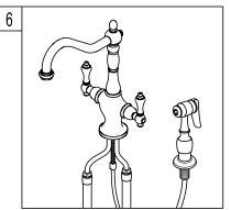
6. Insert the hose through the guide and attach to the fitting on the bottom of the faucet.
